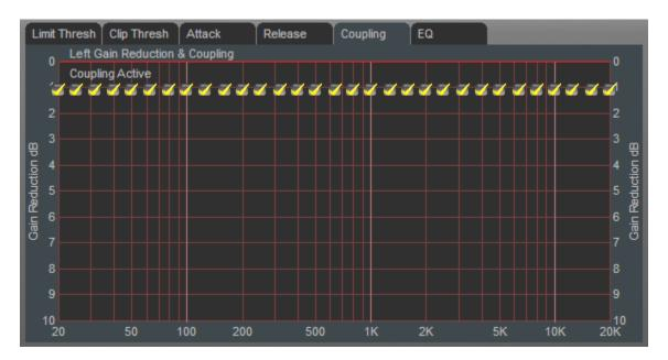
The Coupling controls in the 31 band structure don't couple the control signals from one band to another as is common for the term "coupling", the controls 'hook' or 'unhook' a band from the Wide or Timbral mode when it is running. You cannot unhook a band from Discrete mode!
