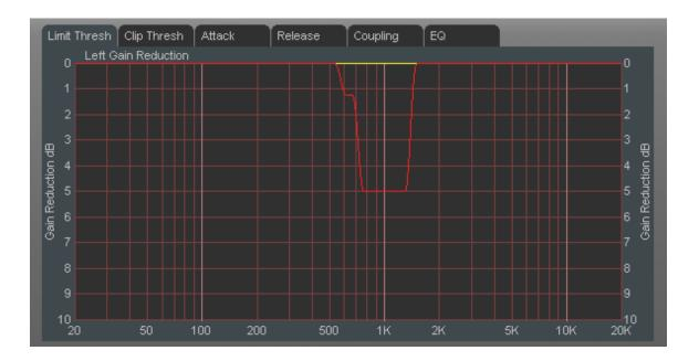
Notice how the range of the frequencies undergoing limiting is wider than in the first example? This is because there are now <u>three</u> bands in limiting even though the 1 kHz tone is present at the center of <u>only</u> the middle band.
