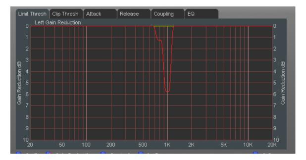
Because there is no limiting at any frequency other than what is required by the 1 kHz tone, any program material that would be near 1 kHz but not high enough to cause its own limiting activity <u>would</u> <u>remain at its original amplitude</u>!
