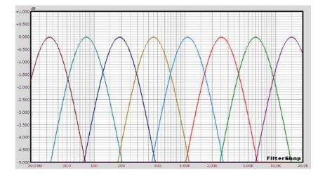
Compare this to the plot below – which is an example of the type of filter bank used in the AP2000 (limited here to just sixteen bands to keep the graphic image clearer).
