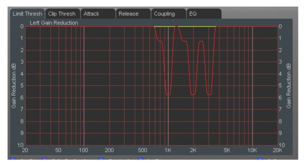
Notice how the 1 kHz band is still in 6dB of limiting but now there is also 6dB of gain reduction occurring in the 2 kHz and 3 kHz bands? This is precisely what the Timbral Mode does – it calculates the harmonics of the primary signal requiring limiting and causes *equal* gain reduction at that frequency as well as its second *and* third harmonics.
