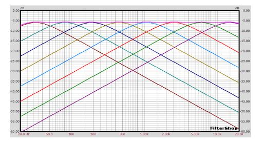
The most important thing to recognize is how <u>broad</u> the crossovers actually are in the eight band example – and the typical four or five band crossover *could* be even broader depending on its design.
