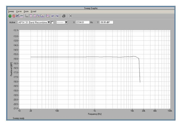
As can be seen from the plot, other than some expected amplitude ripple just prior to the abrupt cutoff of the 15 kHz FM low pass filter the recombined frequency response is virtually flat. And like the frequency response, the phase linearity is also flat with no abrupt departures from linear phase.
